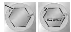
NOTCHING ACTION REDUCE NOTCH PRESURE WITH A CONVENTIONAL KEY. PRESURE WITH A HEX-PLUS® KEY
